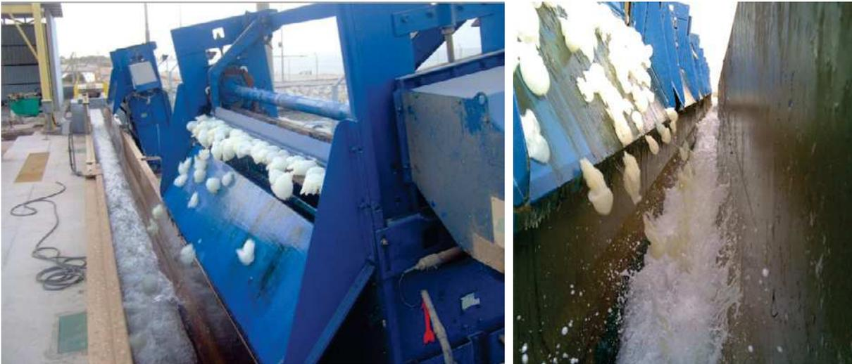
**Figure 3:** Power and MSF-Desalination Plant - Qurrayah, Kingdom of Saudi Arabia. Upgrading with 20 revolving chain screens (by Aqseptence Group), thus removing up to 60 t/h jellyfish per machine out of sea at a total flowrate of 700,000 m<sup>3</sup>/h; material of construction of submerged parts is 316L with impressed current cathodic protection
